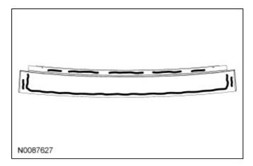
6. Apply the urethane adhesive to the roof glass panel. Follow the pattern as shown.
