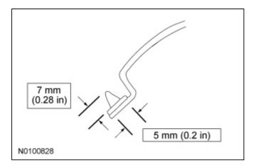
4. **NOTE:** Use either a high-ratio, electric or battery-operated caulk gun that will apply the urethane with less effort and a continuous bead. Make sure there are no gaps in the bead.
