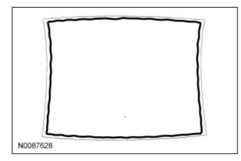
7. **NOTE:** The roof glass applique has a locator pin to make sure of proper fore and aft alignment. The applique must be centered side to side.
