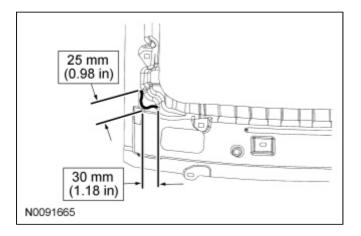
5. Apply the urethane adhesive to the roof glass applique. Follow the pattern as shown.
