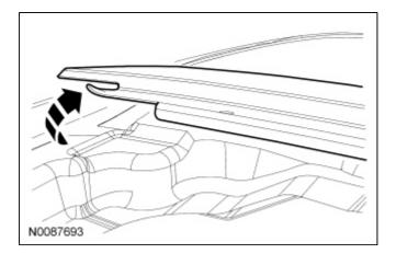
3. **NOTE:** Lubricate the urethane adhesive with water to aid the Deluxe Windshield Removal Tool when cutting the urethane adhesive.
