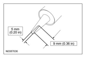
Cut the urethane adhesive applicator tip to specification.
